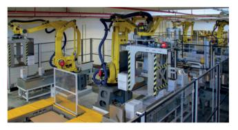
System Logistics responded to this requirement proposing an automated warehouse within the distribution centre in Cerea (Verona), equipped with automatic picking for pallet preparation and fully integrated with the IT logistics systems, thus allowing constant monitoring of warehouse flows. The system is used to supply the Tosano supermarkets and hypermarkets, providing increased efficiency in terms of distribution logistics, with a major impact on cost optimisation and enhanced flexibility.
