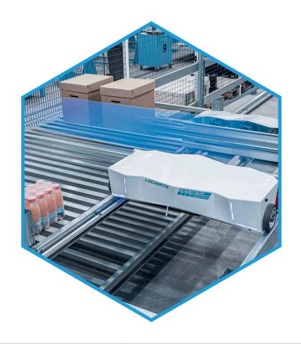
Sequential twin load capability for vehicle job optimization up to 610 x 410 mm
